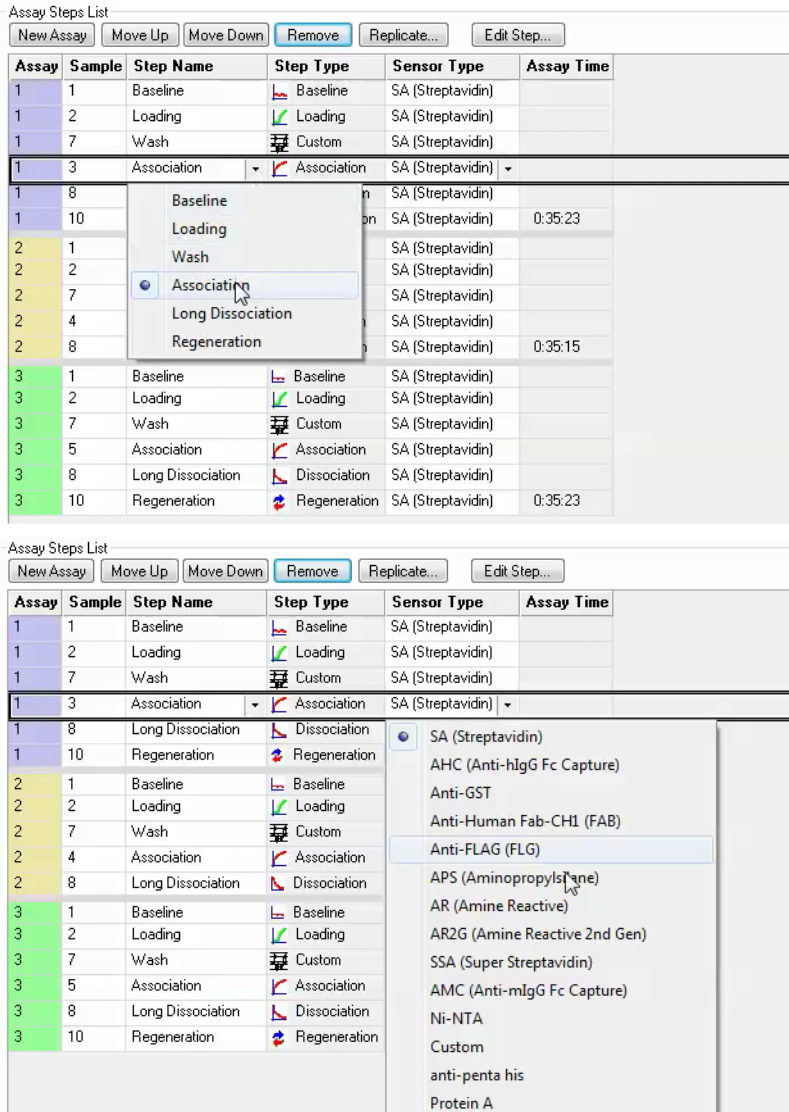
Figure 9-40: Editing an Assay Step Name (top) or Sensor Type (bottom) in the Assay Steps List
